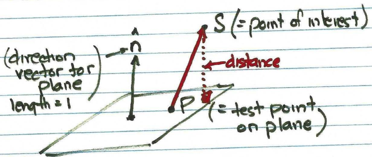
Use ⑮ to get the vector  $\vec{PS}$  from the given co-ordinates of  $S$  and a point  $P$  chosen on the plane. If the equation of the plane (from ⑮) is  $ax + by + cz = d$ , set  $x = y = 0$  and solve for  $z$  to get  $z_0$ .
